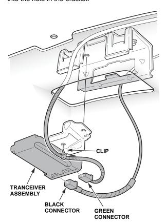
8. Using the bracket bolt removed in step 5, install the transceiver and bracket through the rear individual map light area.
