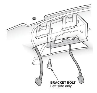
6. Slide the transceiver bracket onto the transceiver.
