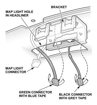
5. Remove the bracket bolt from the bracket.
