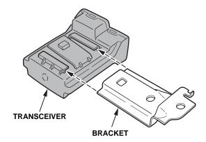
Connect the black and green connector into the transceiver. Then install the clip on the connector into the hole in the bracket.
